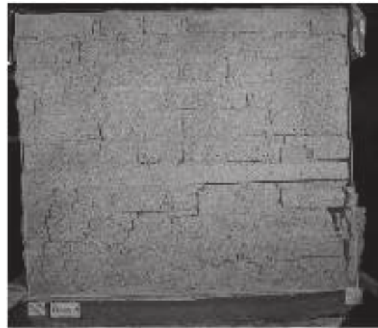
Fig. 14. Wall with timber band at 4560 s of loading at peak displacement towards left.
