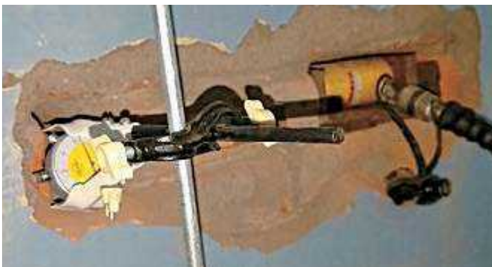
FIGURE 43: IN-SITU PUSH SHEAR TEST TO DETERMINE STRUCTURAL STRENGTH
