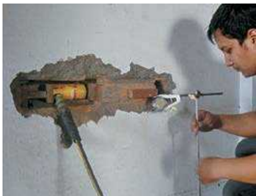
FIGURE 43: IN-SITU PUSH SHEAR TEST TO DETERMINE STRUCTURAL STRENGTH
