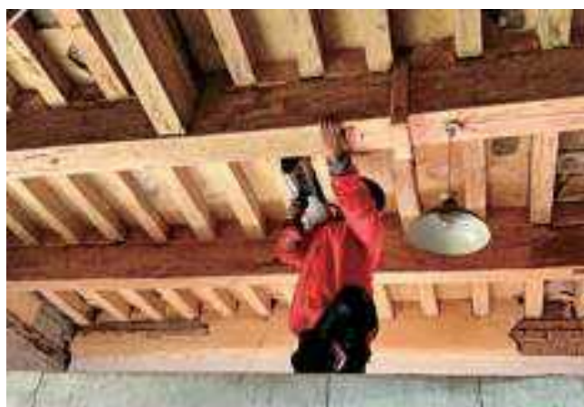
Timber test by Resistor-meter test
